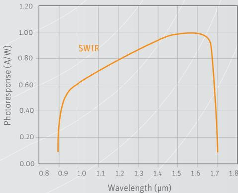
The Bobcat-320 Gated SWIR camera operates in the 0.9 to 1.7 µm spectral band. It provides extremely short integration times down to 100 ns.
